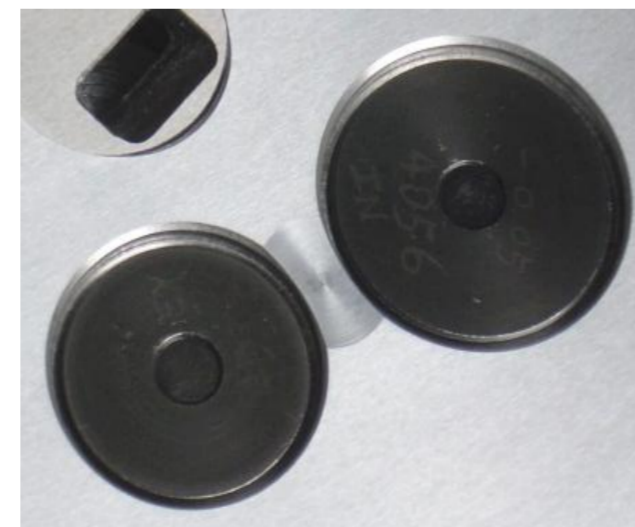
Injectors \varnothing 20mm, Inlet valve \varnothing 40mm, Exhaust valve \varnothing 34mm Valve below the main surface, Inlet & Exhaust valve head recess 1.0 - 1.4mm, square P.C.
