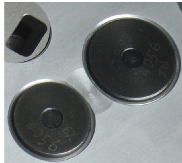
Injectors \varnothing 20mm, Inlet valve \varnothing 40mm, Exhaust valve \varnothing 34mm Valve just out from the main surface, Inlet & Exhaust valve head bulge 0.9 - 1.3mm, square P.C.,
