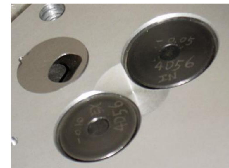
Injectors \varnothing 20mm, Inlet valve \varnothing 40mm, Exhaust valve \varnothing 34mm Valve below the main surface, Inlet & Exhaust valve head recess 1.0 - 1.4mm, round P.C.
