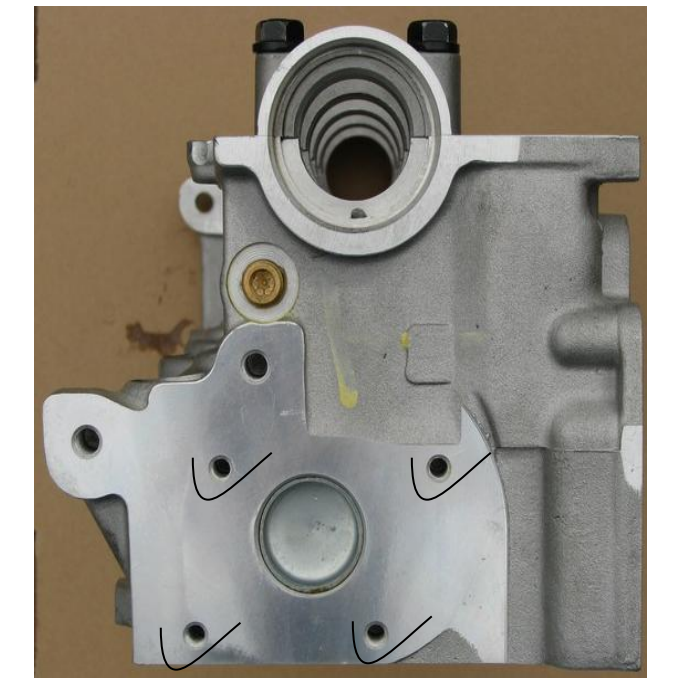
4 Drilled hole to fit water pipe support
